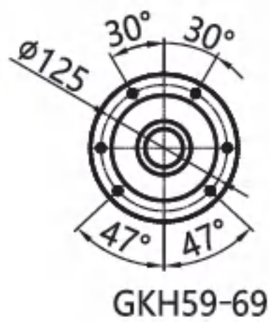
Fig.A Mounting Dimension
